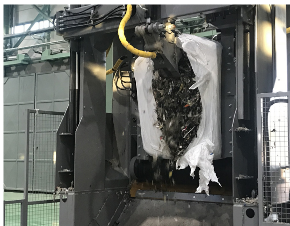
Figure 2. Cross Wrap Bale Opener combines fully automatic, high capacity bale opening with wrapping material removal, together with a robust structure that lasts even in the most demanding surroundings.
