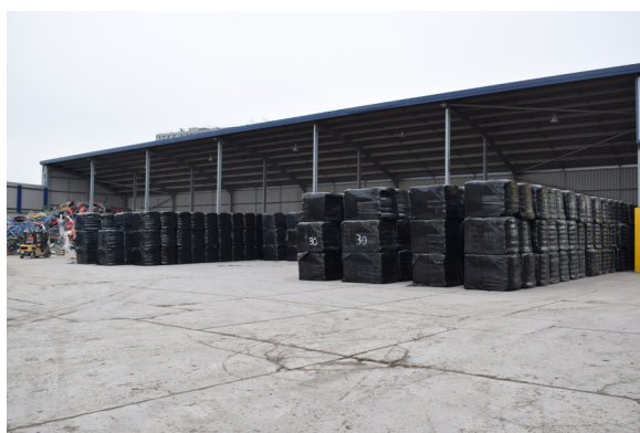
Figure 3. Cross Wrapping the RDF and SRF material offers a clean and cost-effective method for transporting and storing the waste fuels.
