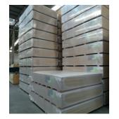
Valuable products with good looking packages attract customers. The machine closes board packages tightly from all six sides using stretch film and bottom skids. The labelling gives the final visual image, helps the operators to handle and recognize the packages in further processes. No straps, covers or bottom pallets are needed.
