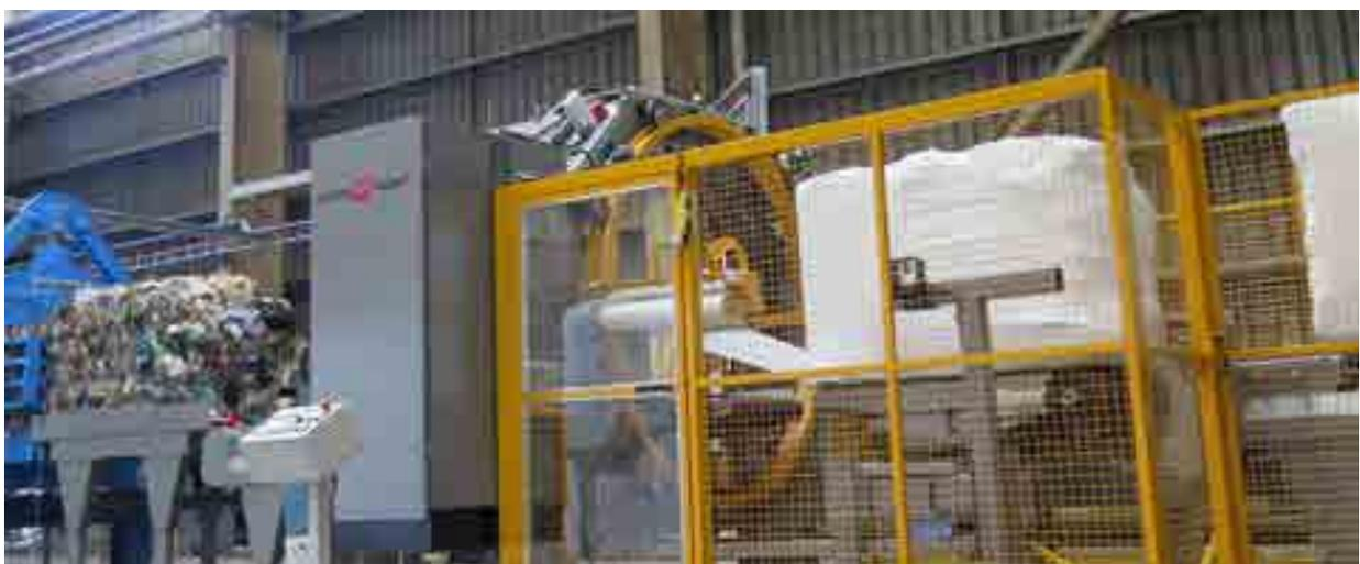
**The Cross Wrap Bale Wrapper at the end of a waste fuel baling line.**
