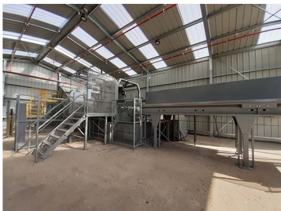
LafargeHolcim Spain invested in an automatic Cross Wrap Bale Opener to improve its waste fuel infeed-operation capacity and process automation.
