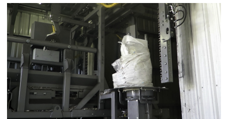
> The wrapping film is removed by the CW 3600 Bale Opener.
