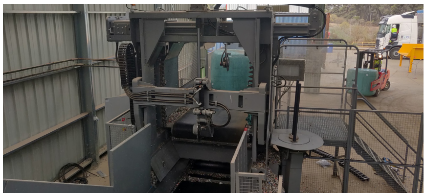
The CW Bale Opener is a fully automatic machine that opens and removes the bale wrap and ties from the baled material.
