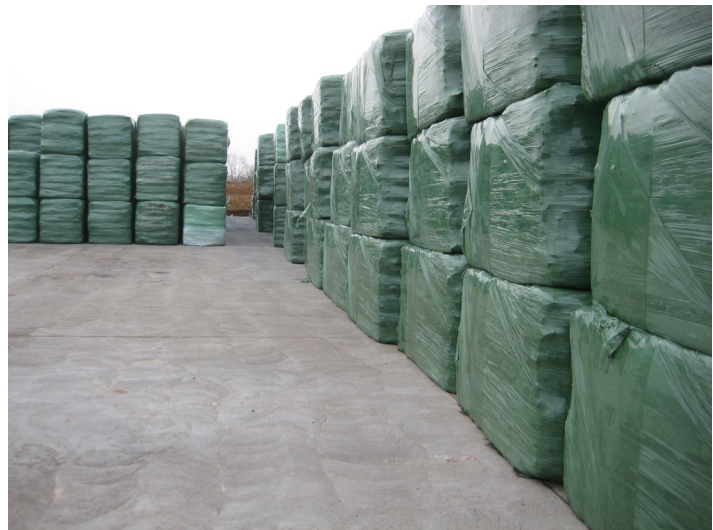
Wrapped alternative fuel bales can be safely stored outside without odours, leakages, or fire risk.
